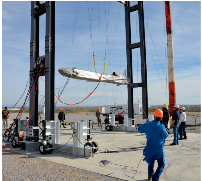
Left: Dozens of off-the-shelf drones are prepared for a systems check at White Sands Missile Range. Above: Engineers lower an Air Force Air Launched Cruise Missile (ALCM) from a frame following a test at White Sands.
